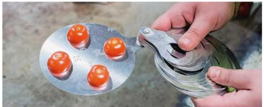
The calibrator, along with the penetrometer, refractometer, thermometer, hygrometer, scales and camera, is one of the most important professional tools of the surveyor
