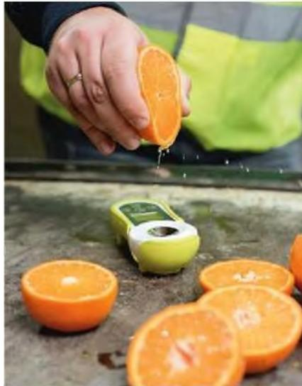
Control of oranges with a portable refractometer
